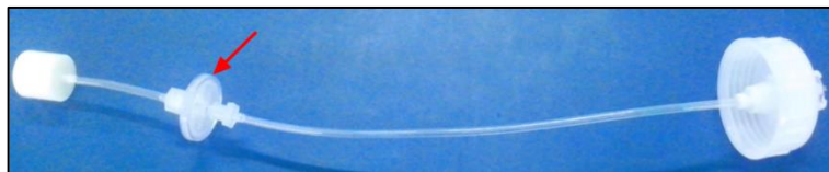
Figure 100. NovoFlow Sheath Fluid Inlet Filter
