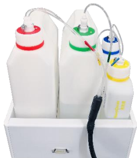
Figure 26. Tubing Connections of the Reagent Containers
