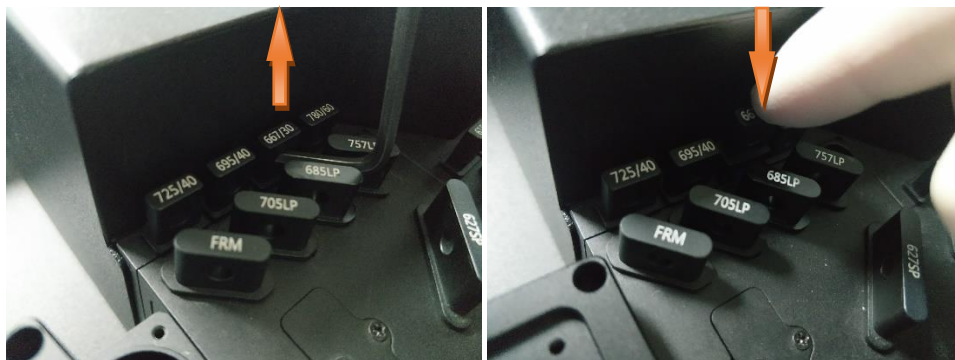
Figure 29. Change the Optical Filter
