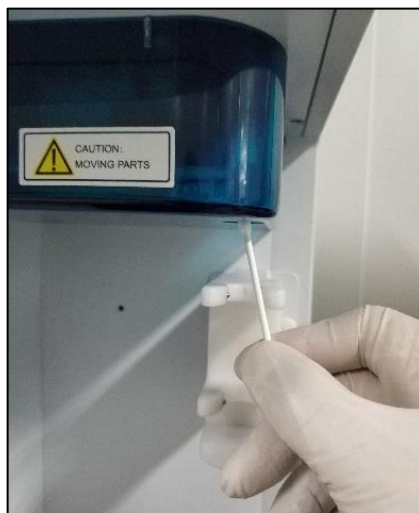
Figure 86. Wipe the SIP Cleaning Apparatus' Lower Surface
